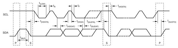
Figure 7. Two-Wire Timing Diagram
