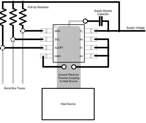
Figure 20. TMP275 Layout Example
