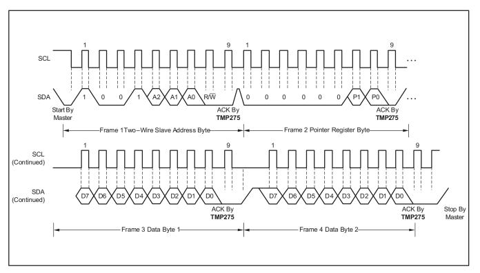
Figure 8. Two-Wire Timing Diagram for TMP275 Write Word Format
