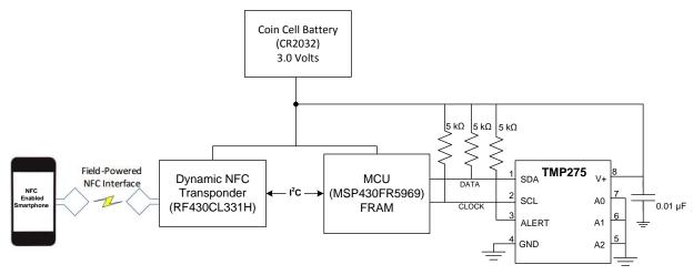
Figure 19. Temperature Data Logger
