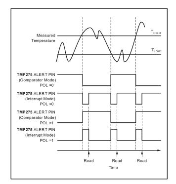
Figure 15. Output Transfer Function Diagrams
