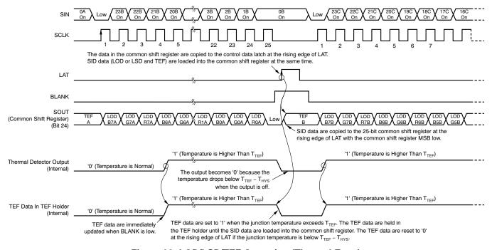
Figure 39. LOD/LSD/TEF Operation (Thermal Error)
