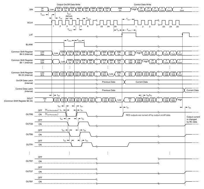
Figure 9. Timing Diagram
