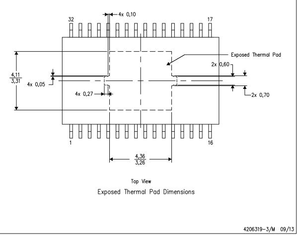
NOTE: All linear dimensions are in millimeters
