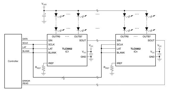
Typical Application Circuit (Multiple Daisy-Chained TLC5952s)
