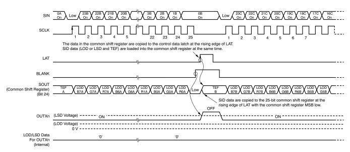
Figure 36. LOD/LSD/TEF Operation (No LED Error)
