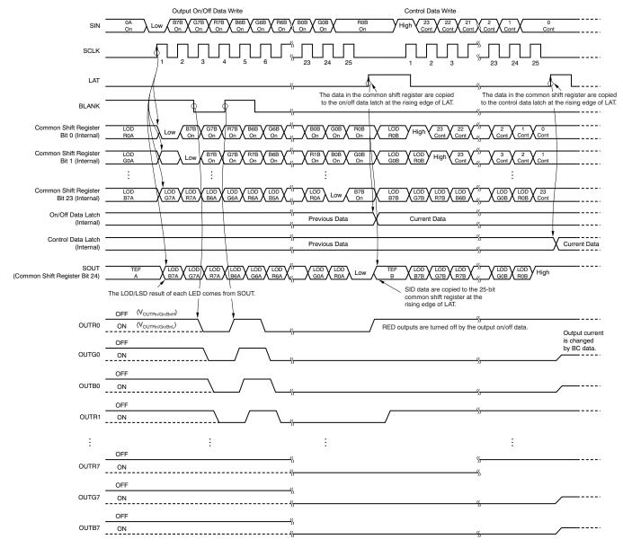
Figure 34. Data Write Operation
