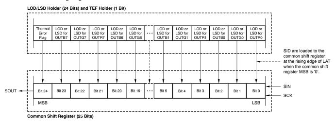
Figure 35. SID Load Assignment
