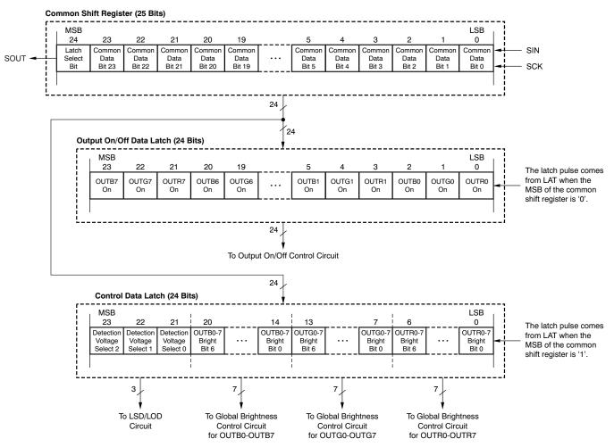
Figure 33. Grayscale Shift Register and Data Latch Configuration
