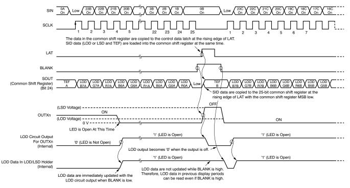
Figure 37. LOD/LSD/TEF Operation (LED Open Error)
