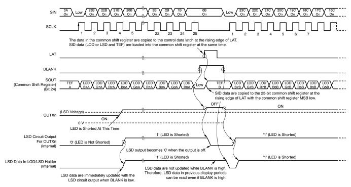
Figure 38. LOD/LSD/TEF Operation (LED Short Error)
