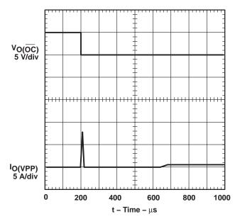
Figure 5. Short-Circuit Response, Short Applied to Powered-on 12-V xVPP-Switch Output
