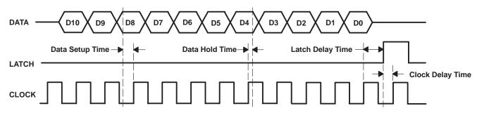
NOTE: Data is clocked in on the positive edge of the clock. The positive edge of the latch signal should occur before the next positive edge of the clock. For definition of D0 to D10, see the control logic table.
