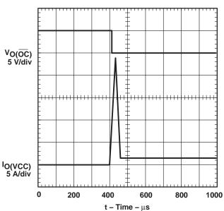
Figure 4. Short-Circuit Response, Short Applied to Powered-on 5-V xVCC-Switch Output
