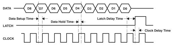
NOTE: Data is clocked in on the positive edge of the clock. The positive edge of the latch signal should occur before the next positive edge of the clock. For definition of D0 to D8, see the control logic table.
