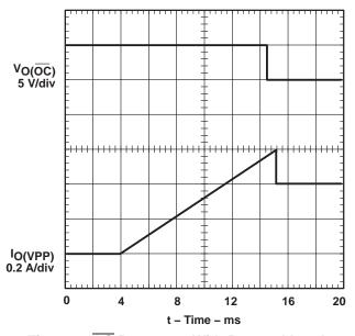
Figure 7. OC Response With Ramped Load on 12-V xVPP-Switch Output
