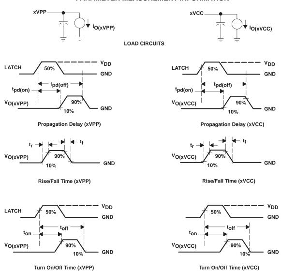
Figure 1. Test Circuits and Voltage Waveforms
