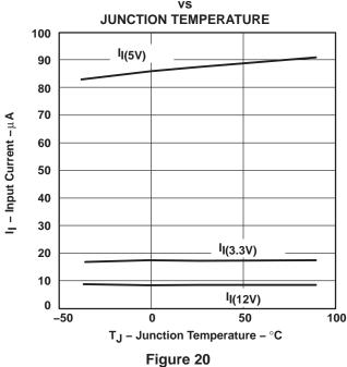
INPUT CURRENT AT  $V_{I(xVCC)} = V_{I(xVPP)} = 5 \text{ V}$ vs
