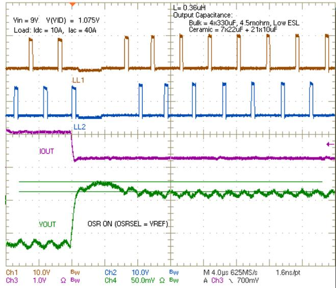
Figure 7. Transient Release Performance Improved with Overshoot Reduction
