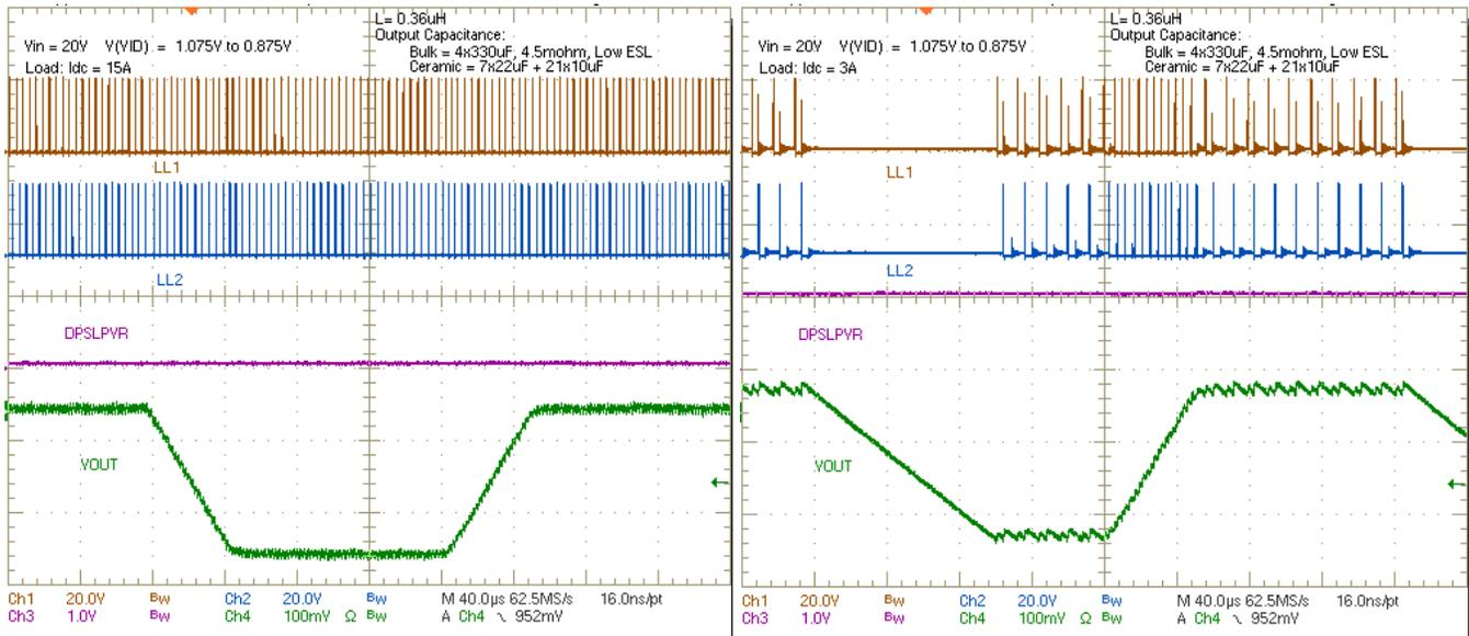
Figure 40. VID Change from 1.075 V to 0.875 V, I<sub>DC</sub> = 15 A
