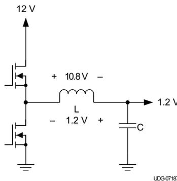
Figure 5. Synchronous Converter
