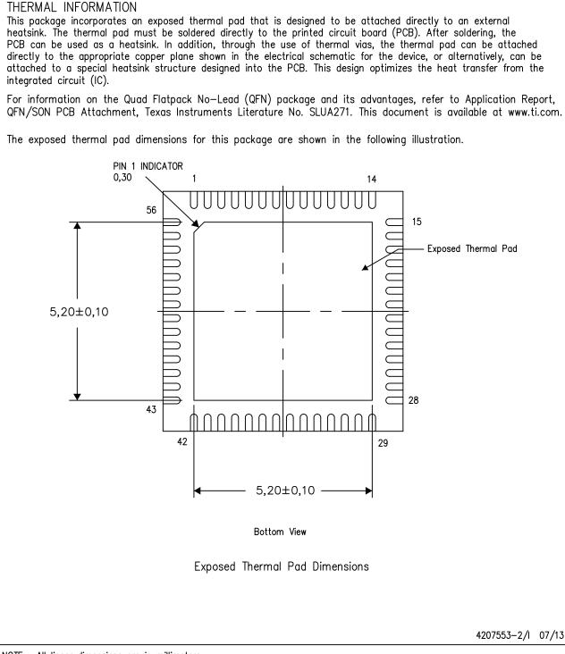
NOTE: All linear dimensions are in millimeters
