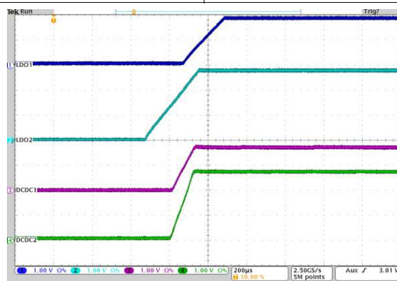
Figure 4-39. Startup DCDC1, DCDC2, LDO1, and LDO2
