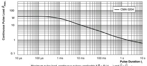
Maximum pulse load, continuous pulses; applicable if  $\vec{P} \le P(\vartheta_{amb})$  and  $\hat{U} \le \hat{U}_{max}$ ; for permissible resistance change equivalent to 8000 h operation
