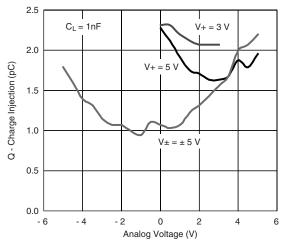
Charge Injection vs. Analog Voltage
