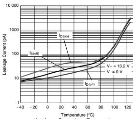
Leakage Current vs. Temperature
