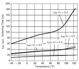
Switching Time vs. Temperature (Single Supply)
