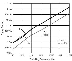
Supply Current vs. Switching Frequency
