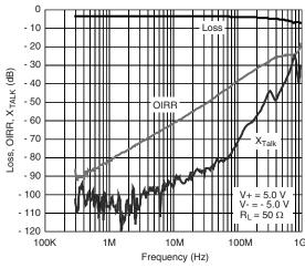
Insertion Loss, Off-Isolation, Crosstalk vs. Frequency
