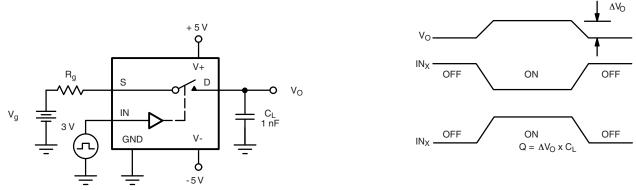
Figure 3. Charge Injection
