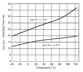
Switching Time vs. Temperature (Dual Supply)
