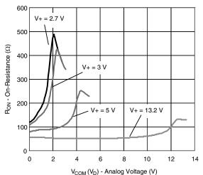
On-Resistance vs. V<sub>D</sub> (Single Supply)
