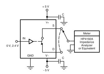
Figure 6. Source/Drain Capacitances
