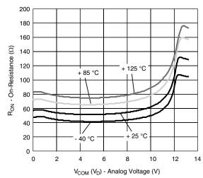
On-Resistance vs. Temperature (Single Supply)
