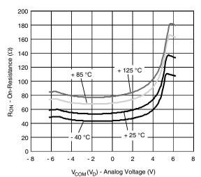
On-Resistance vs. Temperature (Dual Supply)
