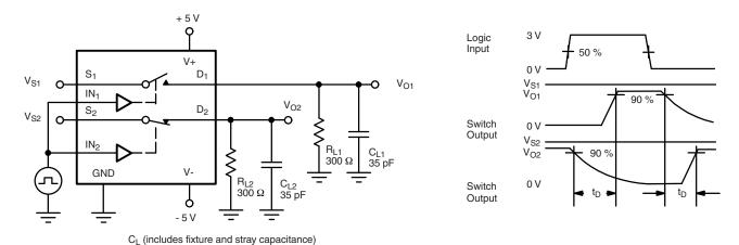
Figure 2. Break-Before-Make (DG613A)
