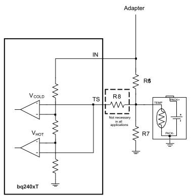
Figure 18. NTC Monitoring Function
