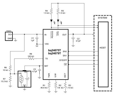
NOTE: V<sub>IN</sub> = UVLO to V<sub>OVP</sub>, I<sub>FASTCHG</sub> = 800mA, I<sub>IN(MAX)</sub> = 1.35A, Battery Temperature Charge Range = 0°C to 50°C, 6.25 hour Fastcharge Safety Timer
