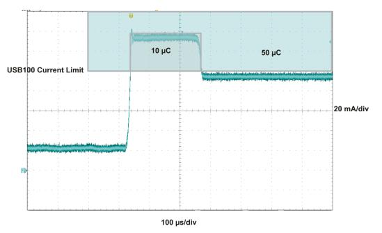
Figure 19. USB-IF Inrush Current Test
