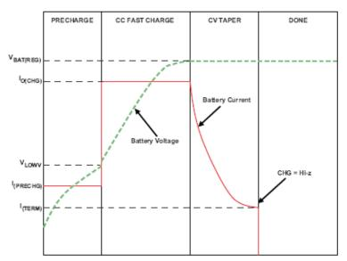
Figure 15. Typical Charging Cycle
