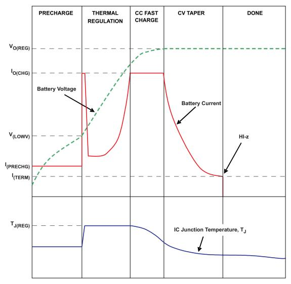
Figure 17. Charge Cycle Modified by Thermal Loop
