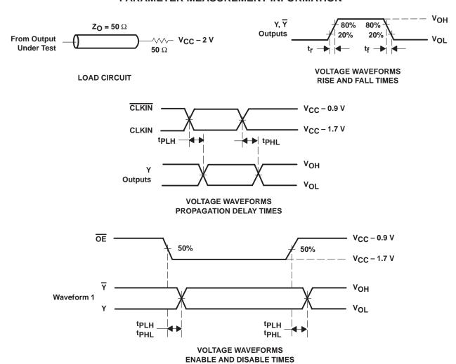
NOTES: A. All input pulses are supplied by generators having the following characteristics: PRR  $\leq$  45 MHz,  $Z_Q = 50~\Omega$ ,  $t_f \leq$  1 ns.  $t_f \leq$  1 ns.
