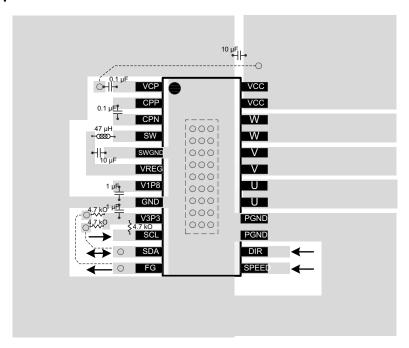
Figure 43. Layout Schematic
