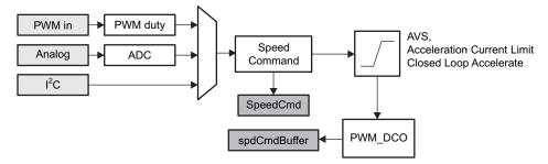
Figure 39. SpeedCmd and spdCmdBuffer Register
