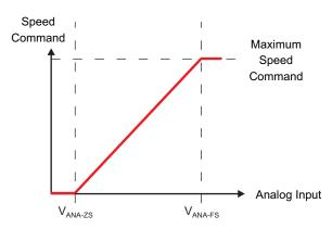
Figure 21. Analog Mode Speed Command
