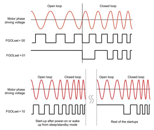
Figure 37. FG Behavior During Open Loop
