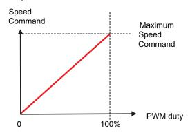
Figure 22. PWM Mode Speed Command
