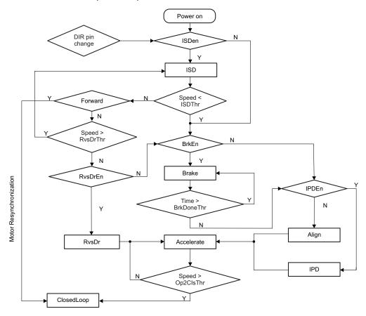
Figure 10. Motor Starting-Up Flow
