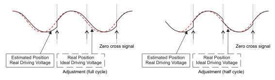
Figure 20. Closed Loop Control Commutation Adjustment Mode
