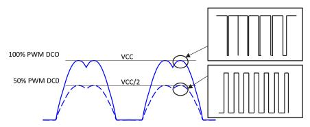
Figure 8. Output Voltage Amplitude Adjustment
