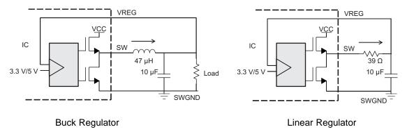
Figure 4. Step-Down Regulator Configurations
