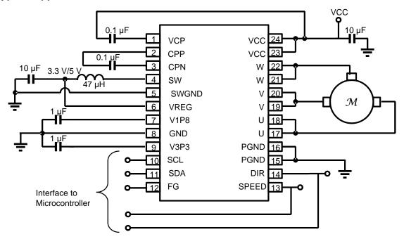
Figure 40. Typical Application Schematic
