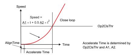
Figure 17. Motor Start-Up Process
