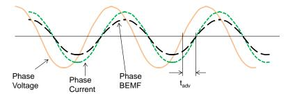
Figure 25. Advance Time (t<sub>adv</sub>) Definition
