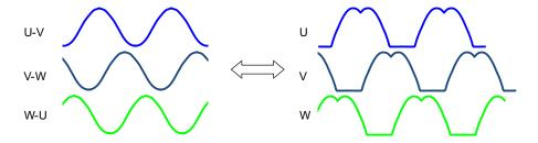
Sinusoidal voltage from phase to phase
