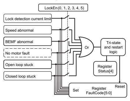
Figure 27. Lock Detect and Fault Diagnose
