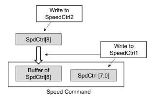
Figure 23. I<sup>2</sup>C Mode Speed Control
