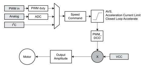
Figure 5. Multiplexing the Speed Command to the Output Amplitude Applied to the Motor
