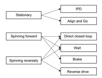
Figure 9. Start the Motor under Different Initial Conditions
