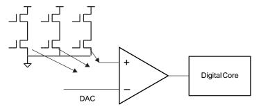
Figure 28. Lock Detection Current Limit
