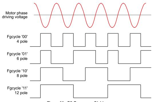
Figure 36. FG Frequency Divider
