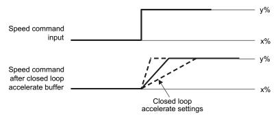
Figure 24. Closed Loop Accelerate
