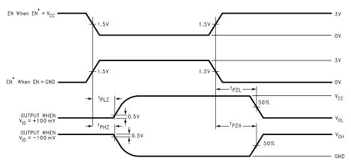
Figure 5. Receiver TRI-STATE Delay Waveforms
