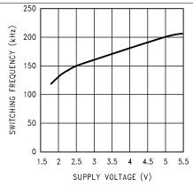
Figure 6. Switching Frequency vs Supply Voltage
