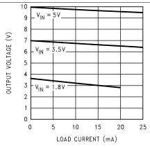
Figure 5. Output Voltage vs Load Current
