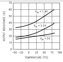
Figure 4. Output Resistance vs Temperature
