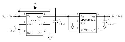
Figure 15. Generate a Regulated 5-V From 3-V Input Voltage
