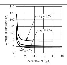
Figure 2. Output Resistance vs Capacitance
