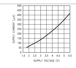
Figure 1. Supply Current vs Supply Voltage
