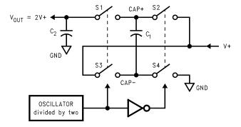
Figure 12. Voltage Doubling Principle
