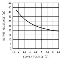
Figure 3. Output Resistance vs Supply Voltage
