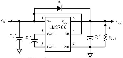
\*  $\mathrm{C_{IN}},~\mathrm{C_{1}}$  , and  $\mathrm{C_{2}}$  are 1.0  $\mu\mathrm{F}$  OS-CON capacitors.
