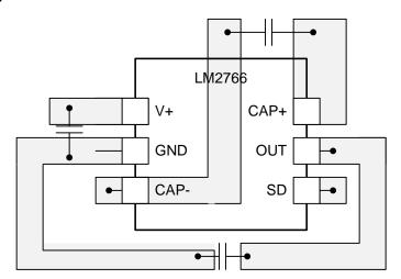
Figure 17. LM2766 Layout Example
