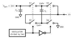
Figure 10. Voltage Doubling Principle
