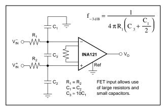
FIGURE 5. Input Low-Pass Filter.
