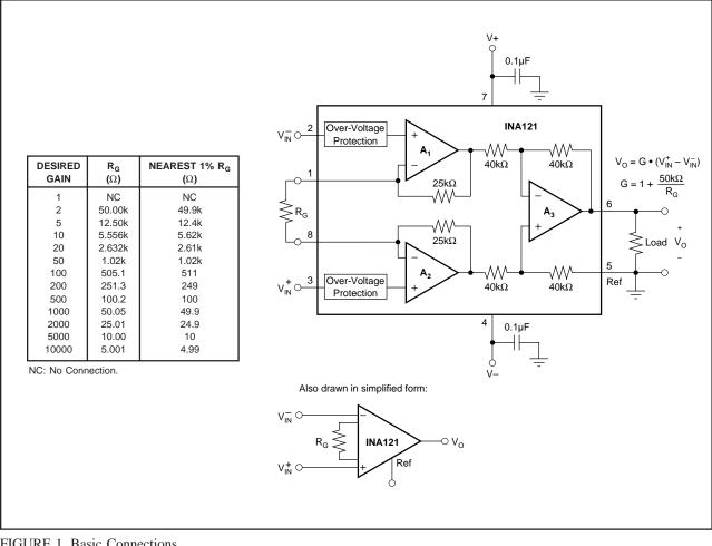
FIGURE 1. Basic Connections.
