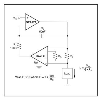
FIGURE 10. Voltage Controlled Current Source.
