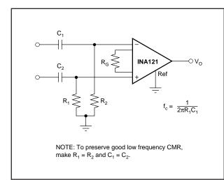
FIGURE 7. High-Pass Input Filter.
