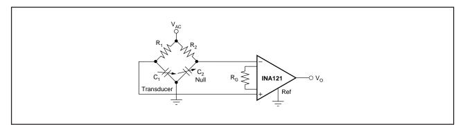
FIGURE 11. Capacitive Bridge Transducer Circuit.
