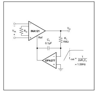
FIGURE 9. AC-Coupled Instrumentation Amplifier.
