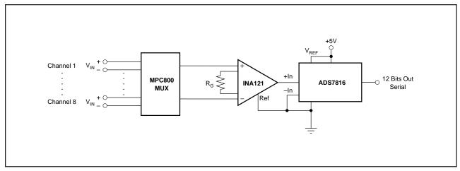
FIGURE 12. Multiplexed-Input Data Acquisition System.
