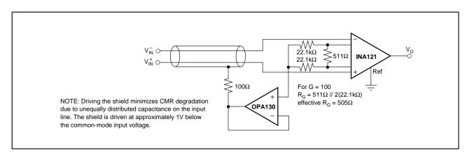
FIGURE 13. Shield Driver Circuit.
