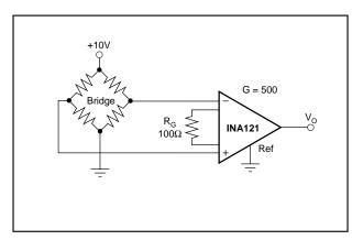
FIGURE 6. Bridge Transducer Amplifier.
