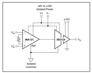
FIGURE 8. Galvanically Isolated Instrumentation Amplifier.
