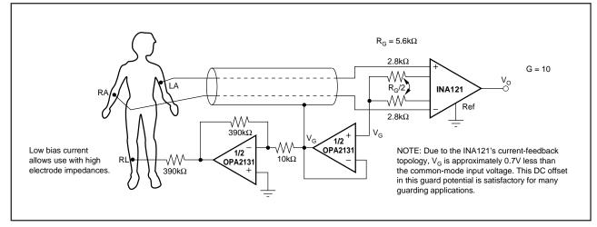
FIGURE 14. ECG Amplifier With Right-Leg Drive.
