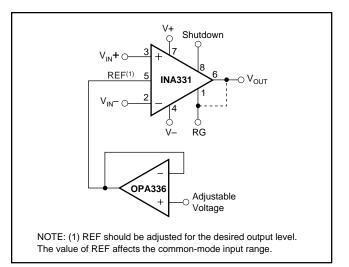
FIGURE 6. Optional Offset Trimming Voltage.
