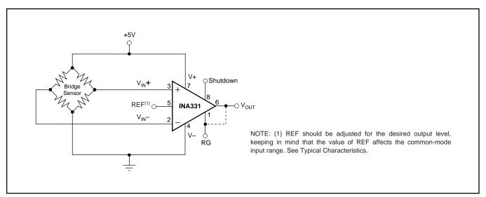
FIGURE 2. Single-Supply Bridge Amplifier.
