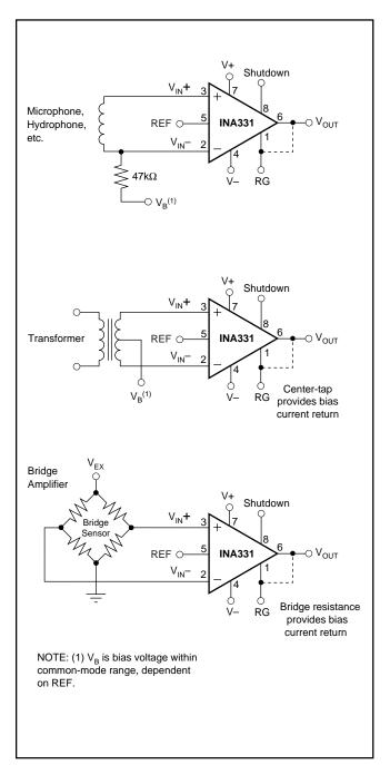
FIGURE 3. Providing an Input Common-Mode Path.
