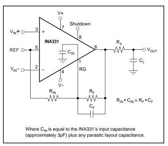
FIGURE 8. Feedback Capacitor Improves Dynamic Performance.
