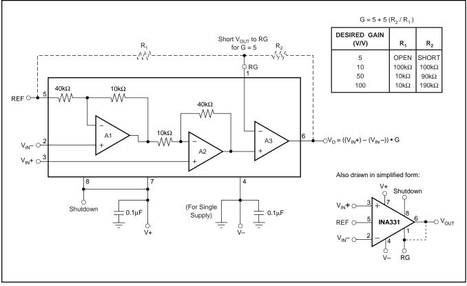
FIGURE 1. Basic Connections.
