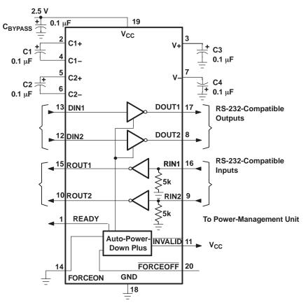
**Figure 5. Typical Application Circuit**
