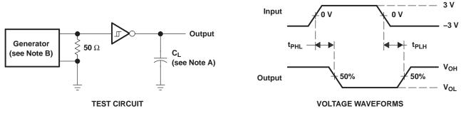
NOTES: A. C<sub>L</sub> includes probe and jig capacitance. B. The pulse generator has the following characteristics:  $Z_O = 50 \Omega$ , 50% duty cycle,  $t_f \le 10$  ns.  $t_f \le 10$  ns.
