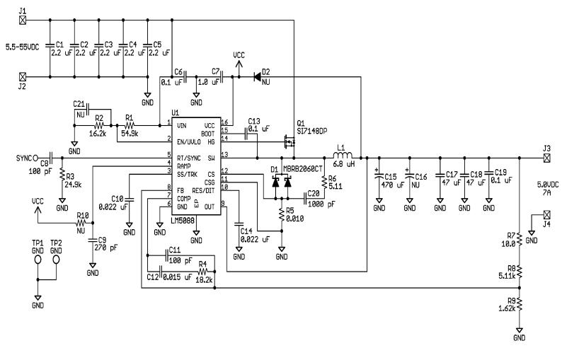
Figure 28. LM5088-2 Application Schematic
