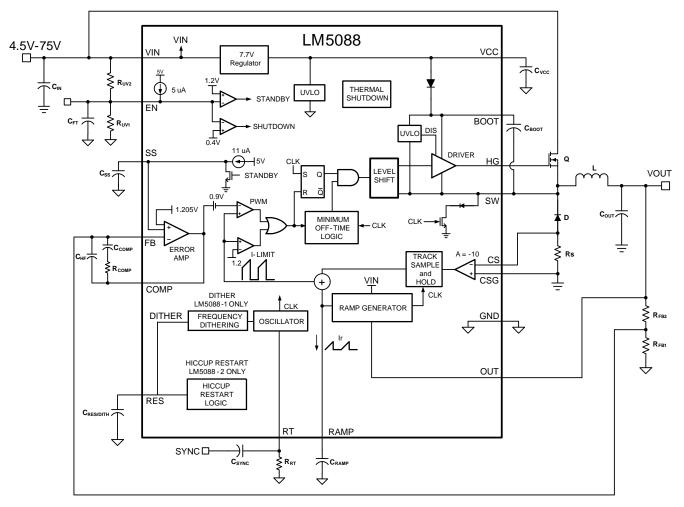
Figure 13. LM5088 Functional Block Diagram
