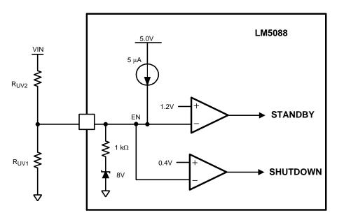
Figure 14. Basic Enable Configuration
