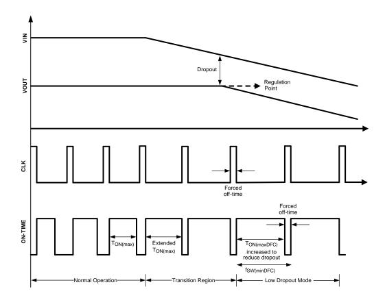
Figure 16. Dropout Voltage Reduction using Dynamic Frequency Control
