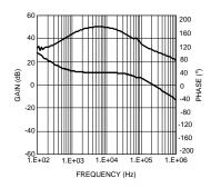
Figure 25. Error Amplifier Gain and Phase
