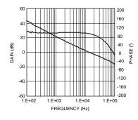
Figure 26. Overall Loop Gain and Phase
