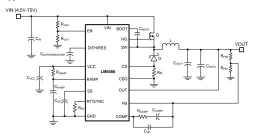
Figure 21. LM5088 Typical Application Schematic
