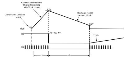
Figure 20. Current Limit Restart Timing Diagram
