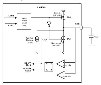
Figure 19. Current Limit Restart Circuit
