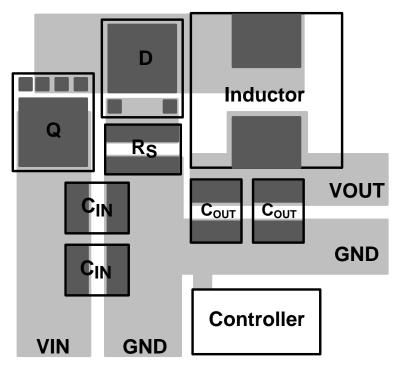
Figure 29. LM5088 Layout Example
