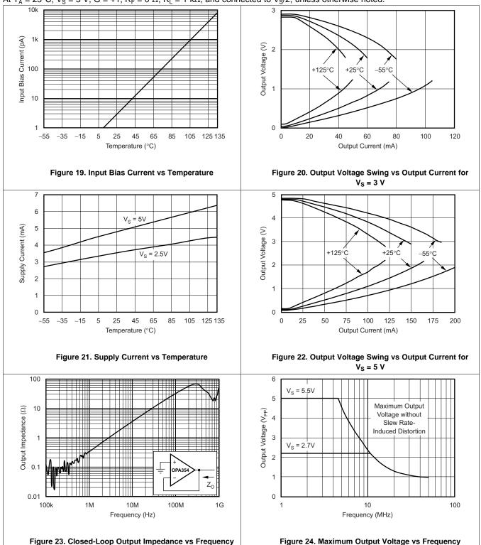
At  $T_A = 25^{\circ}$ C,  $V_S = 5$  V, G = +1,  $R_F = 0 \Omega$ ,  $R_L = 1 k\Omega$ , and connected to  $V_S/2$ , unless otherwise noted.
