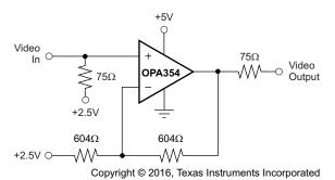
Figure 32. Single-Supply Video Line Driver
