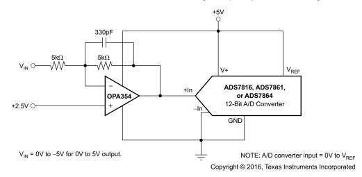
Figure 34. The OPA354 in Inverting Configuration Driving the ADS7816
