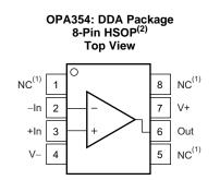
NC means no internal connection.
