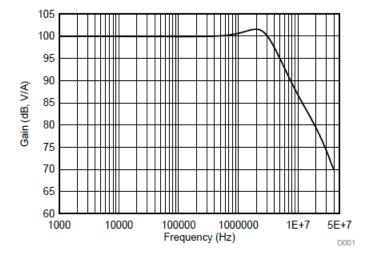
Figure 38. AC Transfer Function
