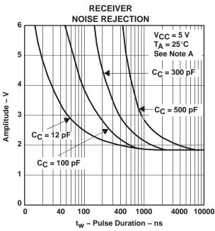
NOTE A: This figure shows the maximum amplitude of a positive-going pulse that, starting from 0, does not cause a change of the output level.
