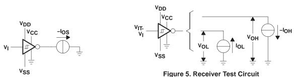
Figure 4. Receiver Test Circuit for IOS
