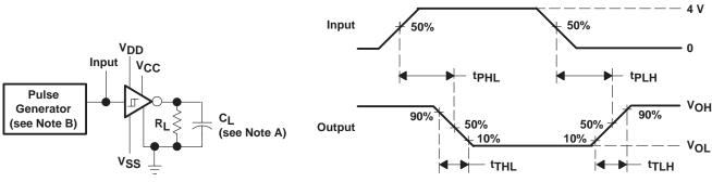
NOTES: A. C<sub>I</sub> includes probe and jig capacitance.
