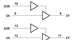
Pin numbers shown are for the D, DB, DGV, J, NS, PW, and W packages.
