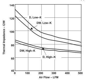
Figure 10. Thermal Impedance vs Air Flow
