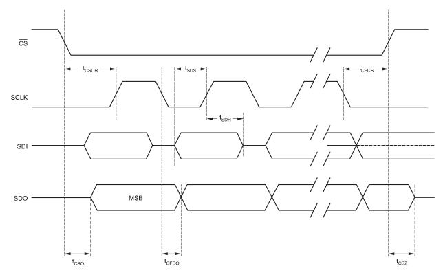
Figure 2. Serial Interface Timing Requirements
