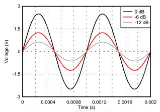
Figure 14. PGA2311 Operating at 0 dB, -6 dB and -12 dB
