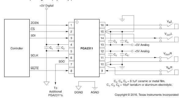
Figure 13. Recommended Connection Diagram
