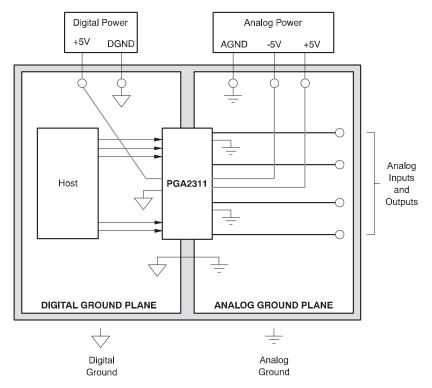
Figure 15. Typical PCB Layout Floor Plan
