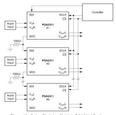
Figure 12. Daisy-Chaining Multiple PGA2311 Devices
