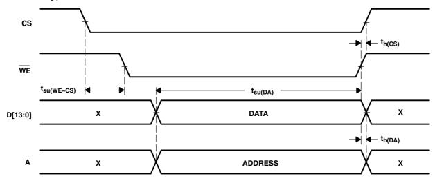
Figure 3. Write Timing
