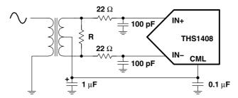
Figure 17. Transformer Coupled
