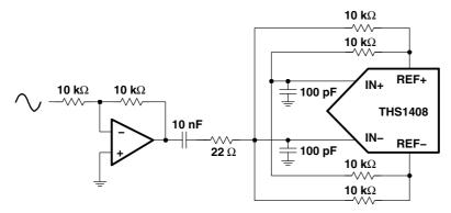
Figure 19. Single-Ended With Level Shift
