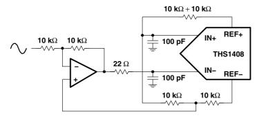
Figure 18. Single-Ended With Level Shift
