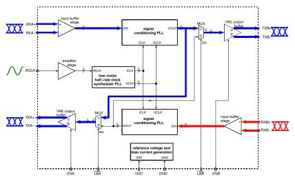
Figure 5. Data Path in Internal Loop-Back Mode A
