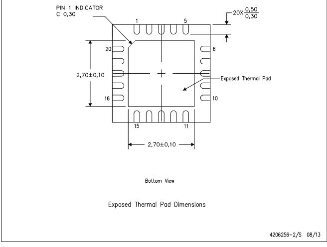
NOTE: All linear dimensions are in millimeters
