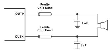
Figure 21. Typical Ferrite Bead Filter (Chip bead example: TDK: MPZ1608S221A)
