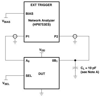
A. C<sub>L</sub> includes probe and jig capacitance.
