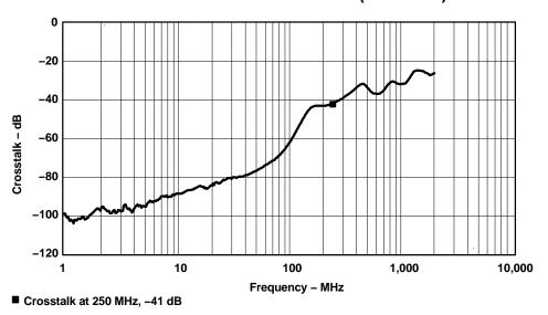
Figure 3. Crosstalk vs Frequency
