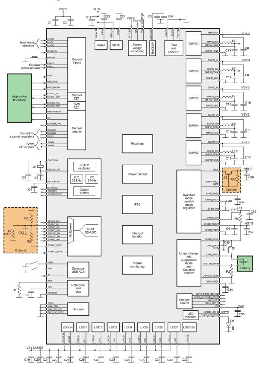
Figure 1-1. TWL6032 Device Block Diagram
