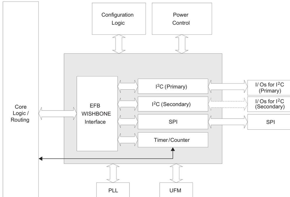
The Platform Manager 2 contains two I<sup>2</sup>C IP cores, the primary and secondary I<sup>2</sup>C IP cores. Each core can be configured either as an I<sup>2</sup>C master or as an I<sup>2</sup>C slave. The main difference between the two IP cores is that the primary core has pre-assigned I/O pin whereas users can assign I/O pins for the secondary core.
