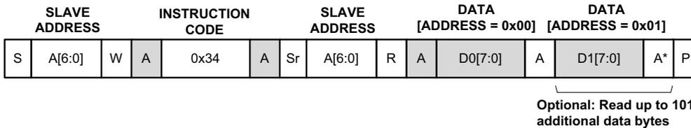
\* After final data byte read, master should NACK before issuing the STOP command
