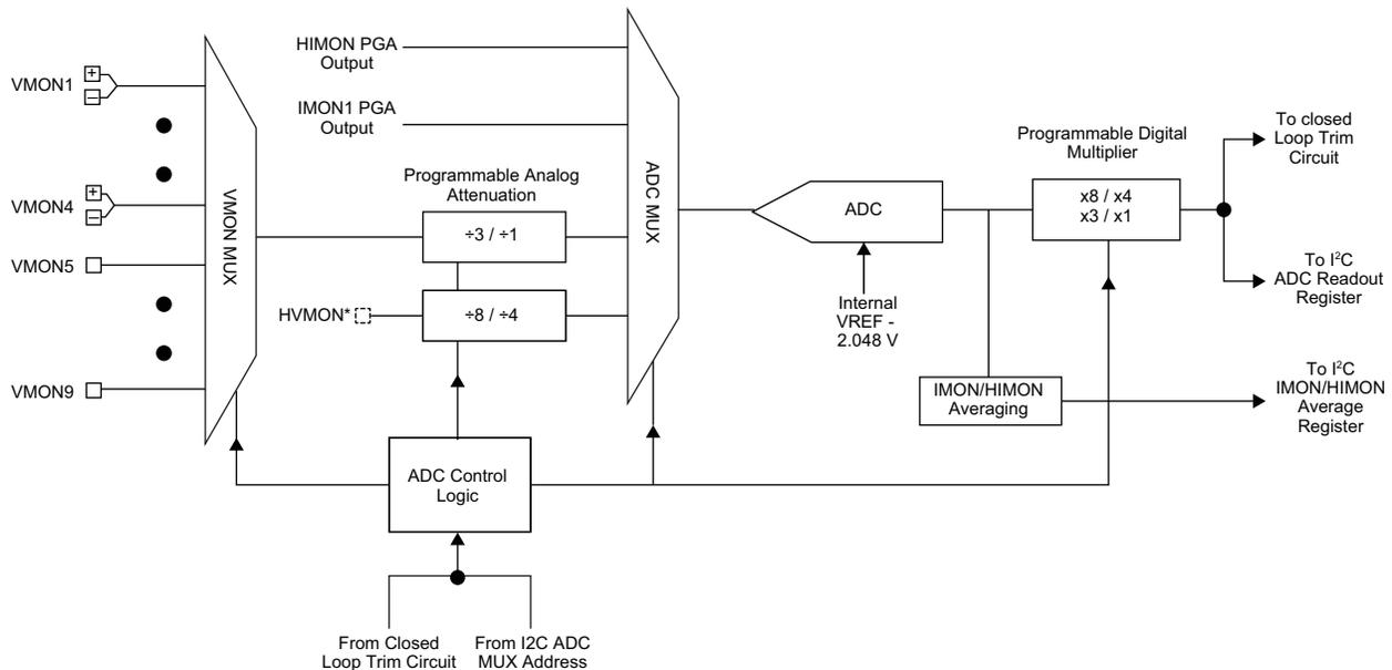
Figure 14 shows the ADC circuit arrangement within the ASC device. The ADC can measure all analog input voltages up to 2.048 V through the multiplexer, ADC MUX. The ADC MUX receives inputs from the High Voltage IMON Programmable Amplifier (PGA), the IMON1 PGA, the High Voltage Monitor (HVMON) at the HIMONN\_HVMON pin, and the VMON MUX. The VMON voltages can be attenuated (divided by three) or unattenuated (divided by
