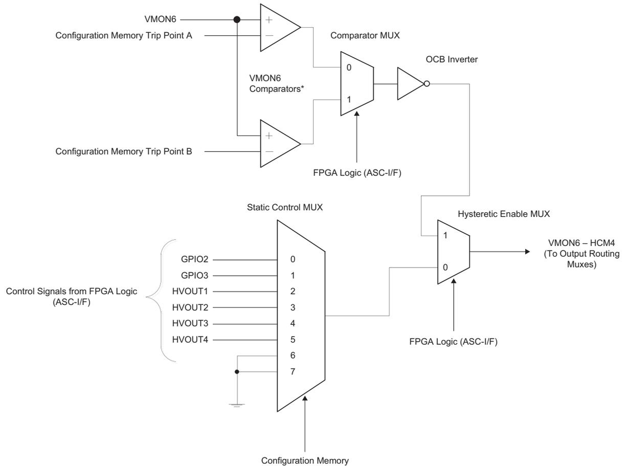
\* VMON6 Windowing and Glitch Filters are not shown in this diagram for clarity. The input to the comparator MUX is from the glitch filters .
