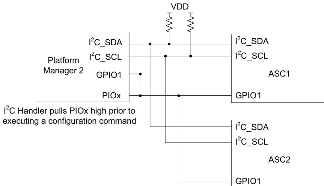
The ASC device will still provide ACK bits in I<sup>2</sup>C write transmissions, even when the configuration write is disabled (by either the GPIO1 state or configuration setting). Even though the device presents ACK bits, the configuration memory will not be overwritten.
