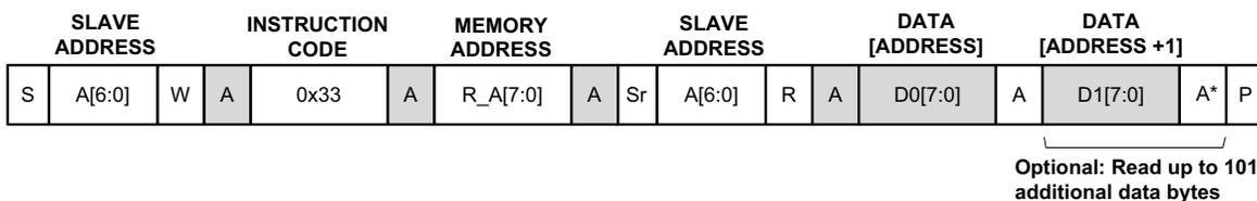
\* After final data byte read, master should NACK before issuing the STOP command.
