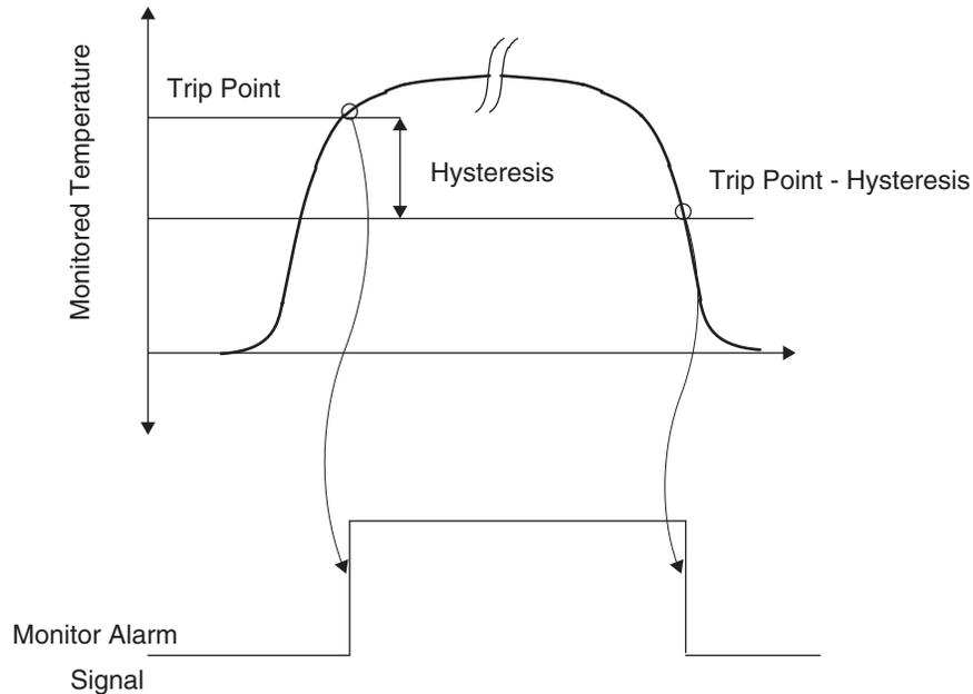
**Figure 18. Monitor Alarm Signal Behavior - Undertemperature (UT) Setting**
