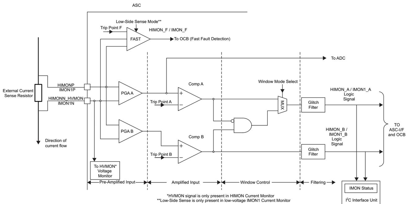
The Current Monitors can be divided into four sections: Pre-Amplified Input, Amplified Input, Window Control, and Filtering. The first section includes the differential input pins IMON1P and IMON1N (low voltage current monitor) or HIMONP and HIMONN\_HVMON (high voltage current monitor). These pins are connected to the PGA circuits as well as the direct differential connection to the Fast Fault Detector.
