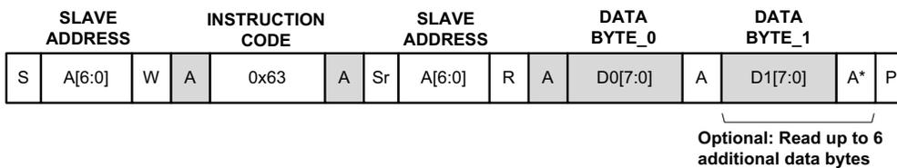
\* After final data byte read, master should NACK before issuing the STOP command
