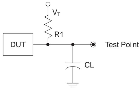
**Table 6. Test Fixture Required Components, Non-Terminated Interfaces**
