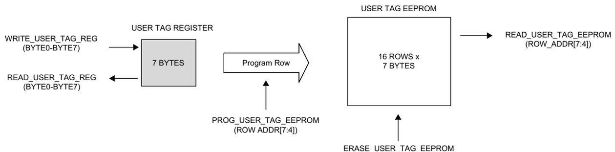
The ERASE\_USER\_TAG\_EEPROM instruction is used to erase the entire User Tag EEPROM array. The User Tag can only be erased as a full block. A row must be erased prior to programming it. The instruction format for ERASE\_USER\_TAG\_EEPROM is shown in Figure 63.
