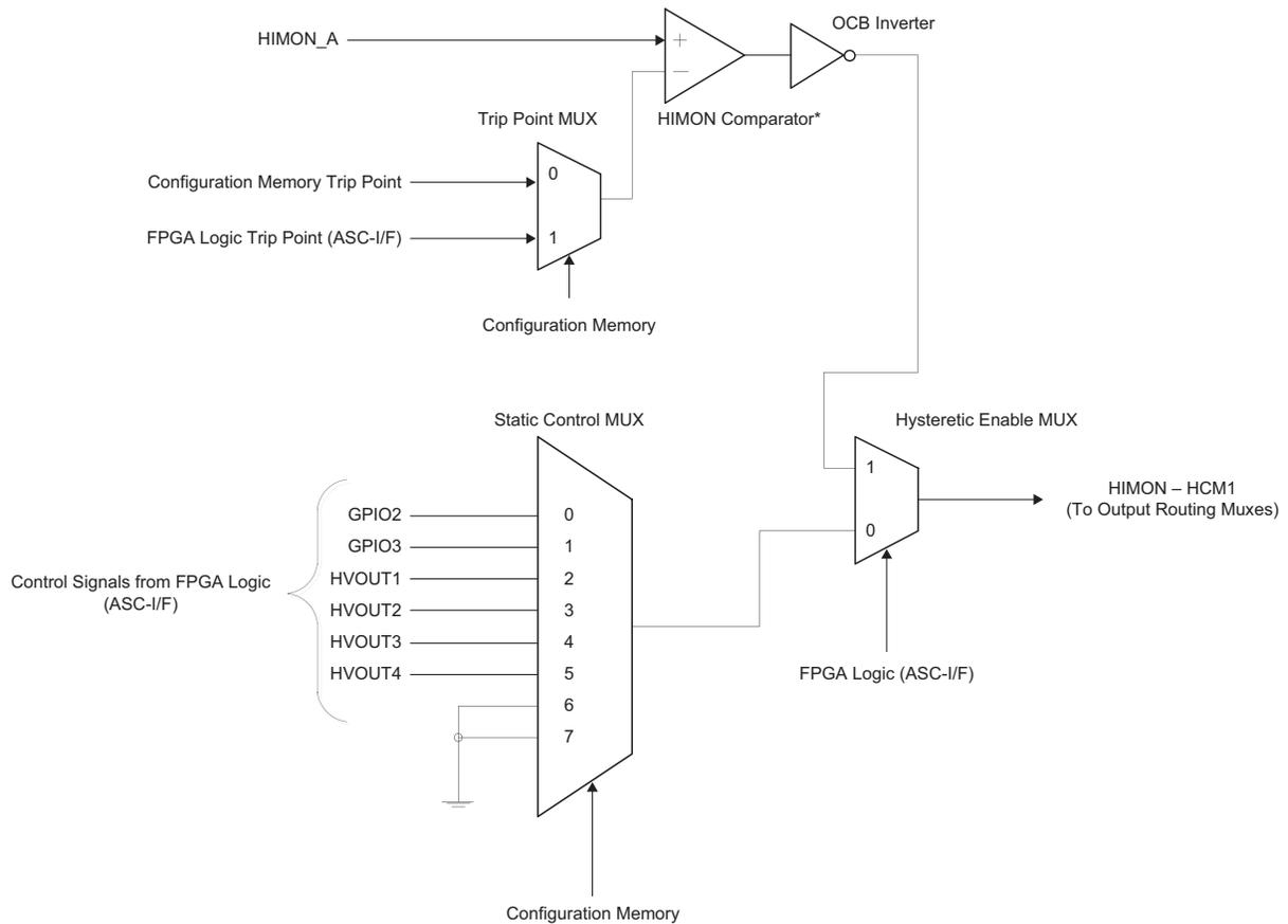
\* HIMON Windowing and Glitch Filters are not shown in this diagram for clarity. The input to the OCB inverter is from the glitch filter.
