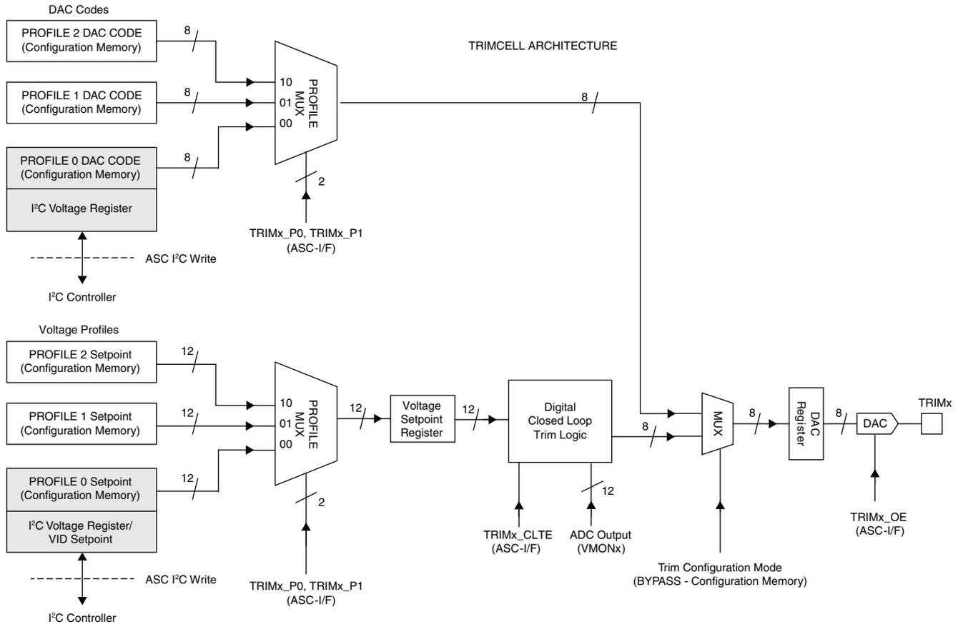
Profile0, Profile1 and Profile2 are 12-bit setpoints, which are written in the EEPROM memory during programming. The active profile for each TrimCell is independently chosen based on ASC-I/F signals TRIMx\_P0 / TRIMx\_P1. This profile is copied to the Voltage Setpoint Register whenever the TRIMx\_P0, TRIMx\_P1 signals change.
