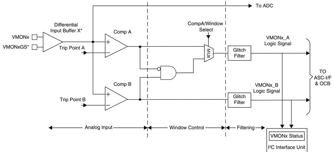
\*Differential Input Buffer X and VMONxGS pins are not present for single-ended VMON x inputs.
