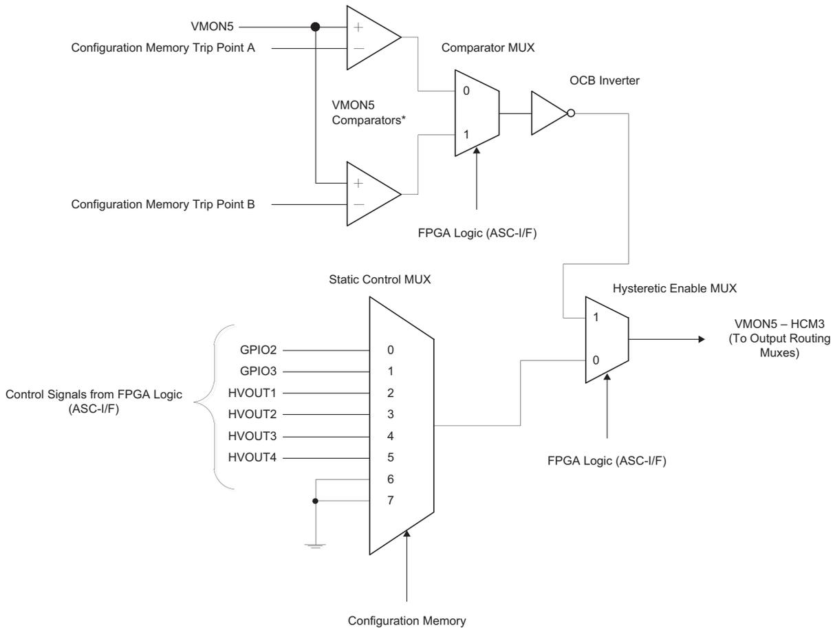
\* VMON5 Windowing and Glitch Filters are not shown in this diagram for clarity. The input to the comparator MUX is from the glitch filters.
