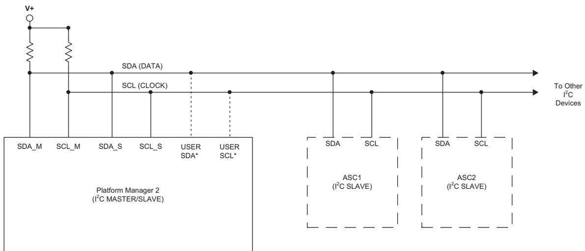
\* - Adding a USER\_SDA and USER\_SCL is application dependent and not required for all systems. This port is for accessing FPGA logic resources over I<sup>2</sup>C.
