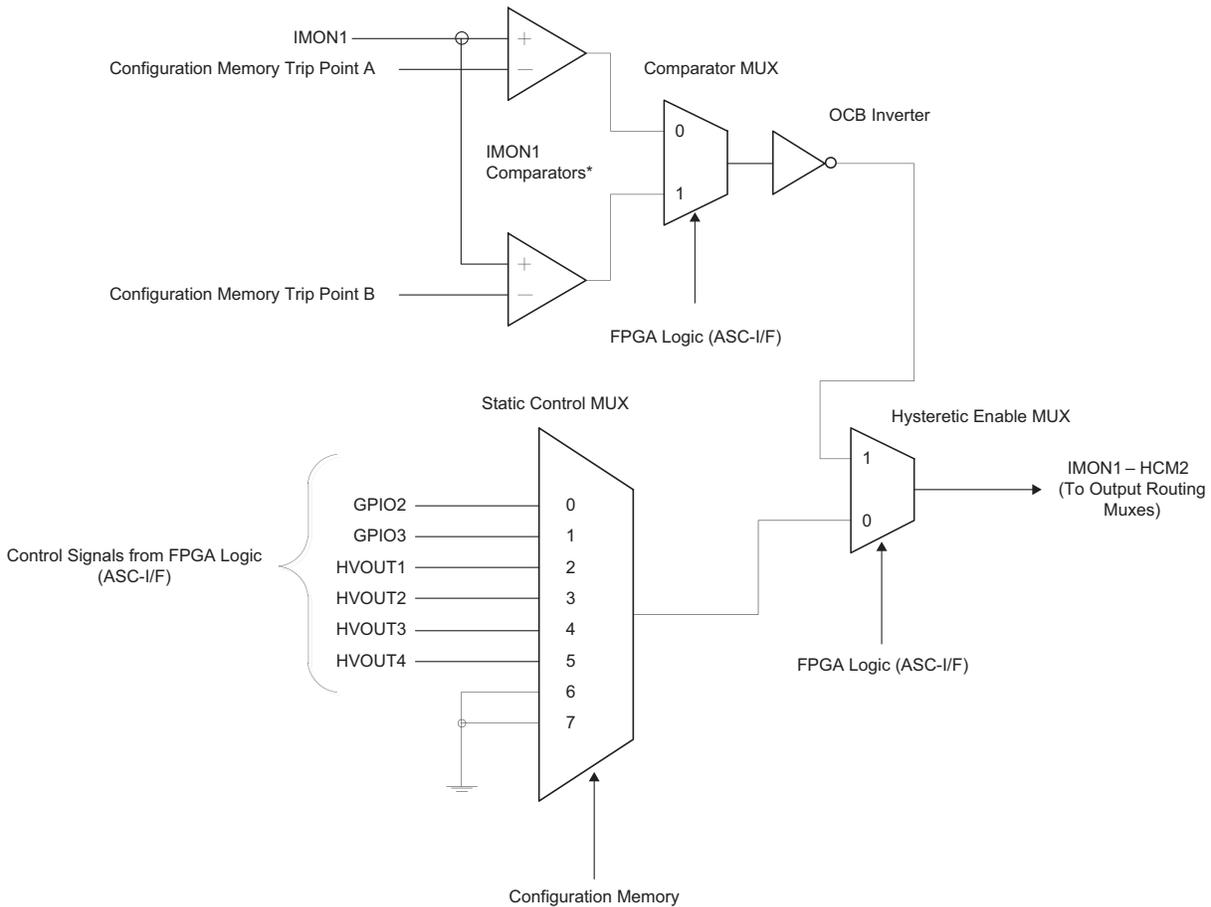
\* IMON Windowing and Glitch Filters are not shown in this diagram for clarity. The input to the comparator MUX is from the glitch filters.
