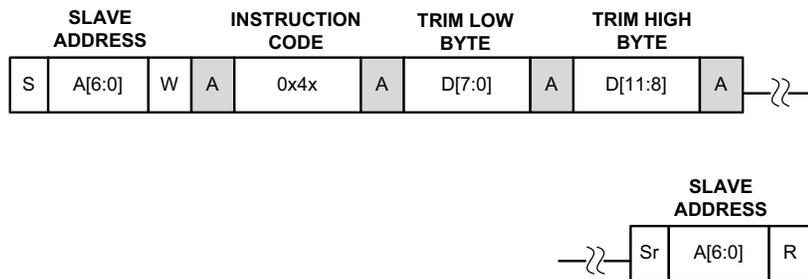
The new trim target will be latched in the hardware at the completion of this sequence.
