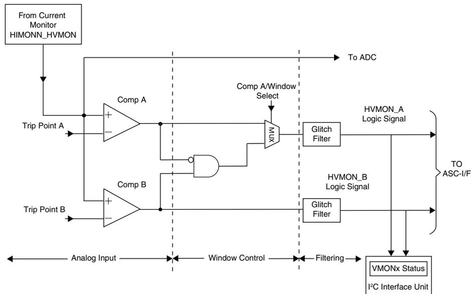
The HVMON follows the same structure as the Voltage Monitor circuits. Two individually programmable trip-point comparators are connected to the HIMONN\_HVMON pin voltage. Each of the comparator references has 408 programmable trip points, over a range of 0.227 V to 13.226 V.
