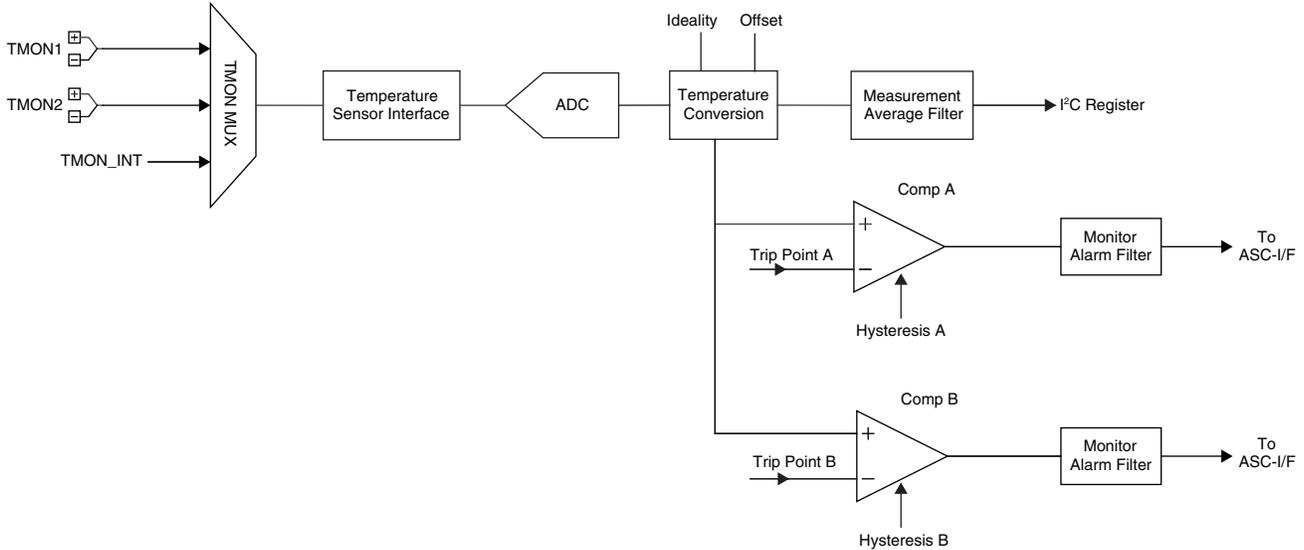
The independently programmable temperature monitor inputs can be used with internal substrate diodes on microprocessors, FPGAs, ASICs, or with low cost external NPN or PNP transistors. The temperature sensor interface block includes programmable support for a variety of sensor configurations as shown in Figure 16. The sensor configuration settings available in the design software are described in Table 13.
