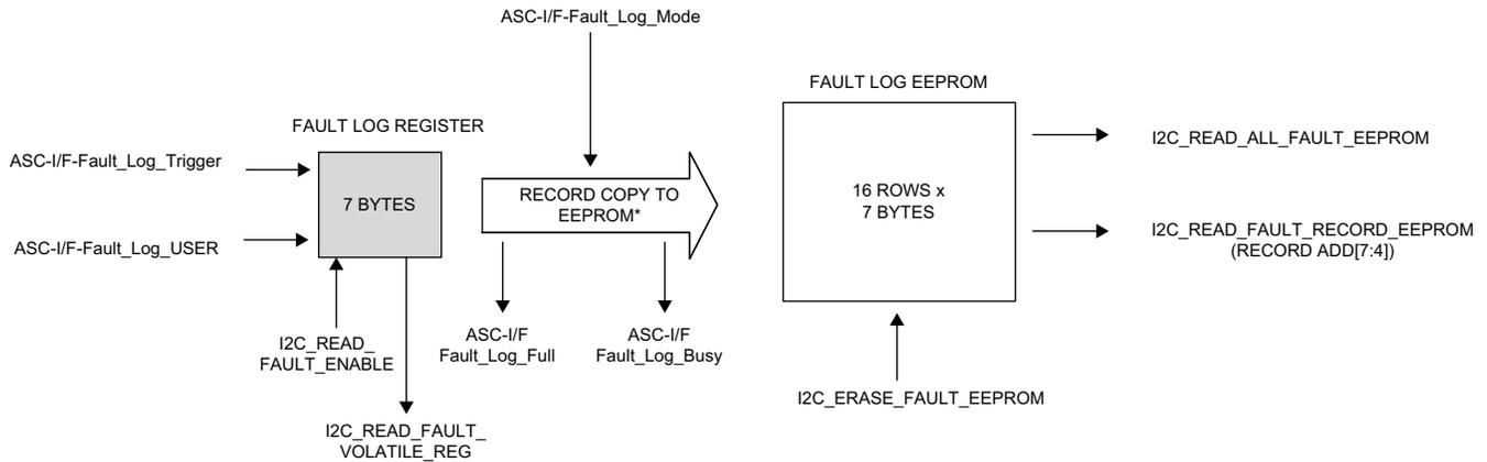
\* - Fault Log record programming number is automatically incremented each time a fault log is recorded in the memory. The next programming row is recorded in the status register, accessed by the READ\_STATUS I2C command.
