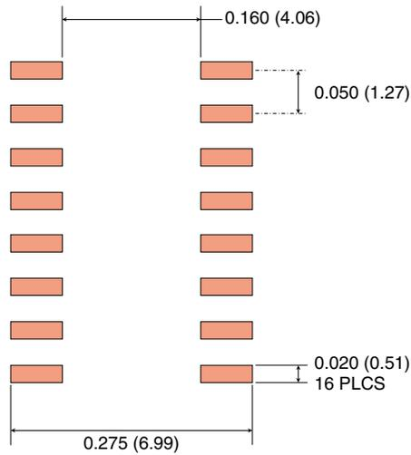
**0.3" 16-pin SOIC Pad Layout**
