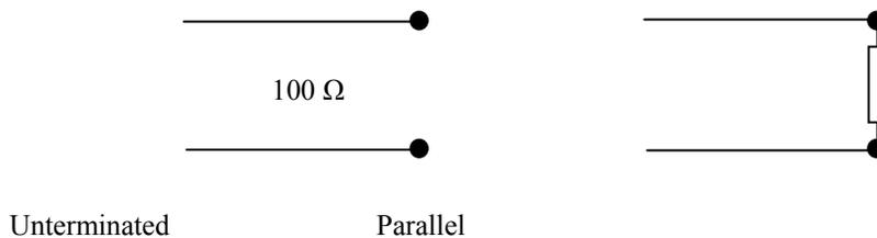
Proper termination is imperative when using IL3285 and IL3222 to minimize reflections. Unterminated lines are only suitable for very low data rates and very short cable runs, otherwise line reflections cause problems. Parallel terminations are the most popular. They allow high data rates and excellent signal quality.
