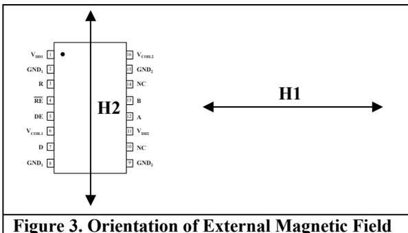
An applied field in the direction of “H2” has considerably less effect on the sensor and will result in significantly higher immunity levels as shown in Table 1.
