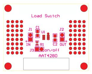
Figure 1: AAT4280 Evaluation Board Top Side Silk Screen Layout / Assembly Drawing.
