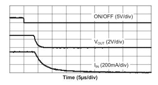
AAT4280-3 Turn-Off  $(V_{IN} = 5V; R_L = 10\Omega)$
