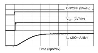
AAT4280-2 Turn-On  $(V_{IN} = 5V; R_L = 10\Omega)$
