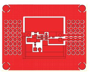
Figure 2: AAT4280 Evaluation Board Component Side Layout.
