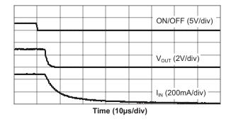
AAT4280-1 Turn-Off  $(V_{IN} = 5V; R_L = 10\Omega)$
