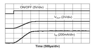
AAT4280-1 Turn-On  $(V_{IN} = 5V; R_L = 10\Omega)$
