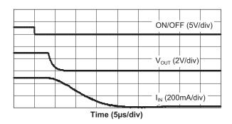
AAT4280-2 Turn-Off  $(V_{IN} = 5V; R_L = 10\Omega)$
