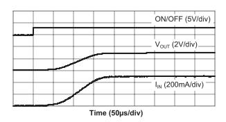
AAT4280-3 Turn-On  $(V_{IN} = 5V; R_L = 10\Omega)$
