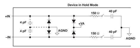
Figure 51. Input Equivalent Circuit
