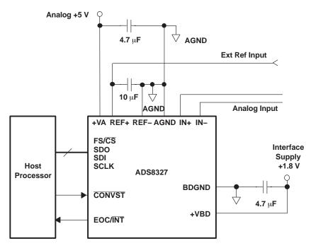
Figure 66. Typical Circuit Configuration
