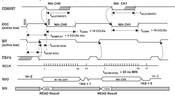
Figure 6. Simplified Dual Channel Timing
