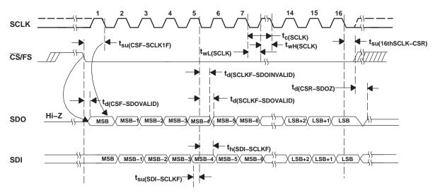
Figure 5. Detailed SPI Transfer Timing
