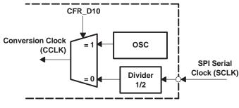
Figure 54. Converter Clock
