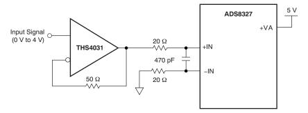
Figure 52. Unipolar Input Drive Configuration
