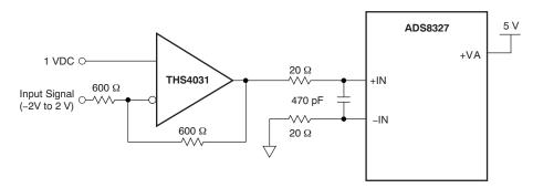
Figure 53. Bipolar Input Drive Configuration
