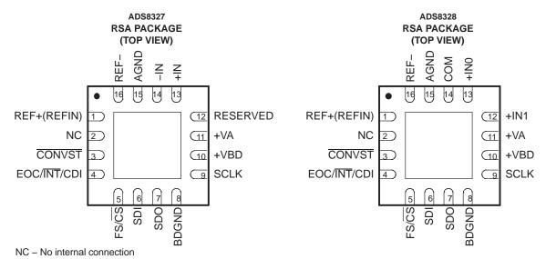
**CAUTION:** The thermal pad is internally connected to the substrate. This pad can be connected to the analog ground or left
