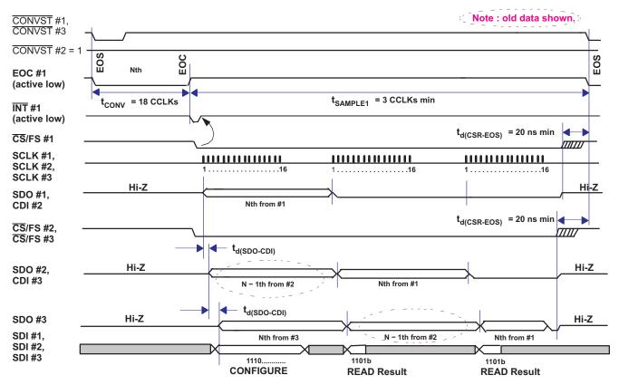
Figure 62. Simplified Cascade Timing (Separate CONVST)
