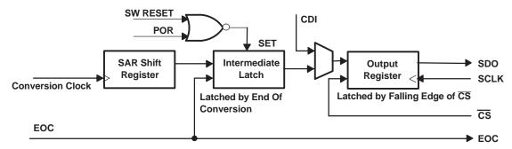
Figure 64. Digital Output Under Reset Condition
