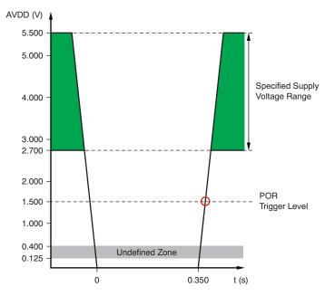
Figure 65. Relevant Voltage Levels for POR
