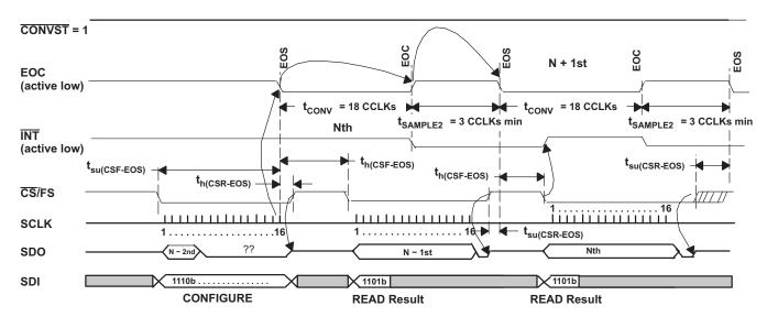
Figure 4. Timing for Conversion and Acquisition Cycles for Autotrigger (Read While Converting)
