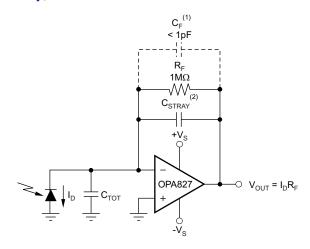
NOTES: (1)  $C_F$  is optional to prevent gain peaking. (2)  $C_{STRAY}$  is the stray capacitance of  $R_F$ (typically, 2pF for a surface-mount resistor). Copyright © 2016, Texas Instruments Incorporated
