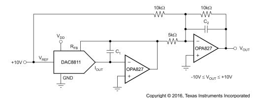
Figure 51. I/V Converter
