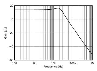
Figure 49. OPA827 Second-Order, 25-kHz, Chebyshev, Low-Pass Filter
