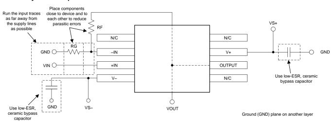
Figure 52. Operational Amplifier Board Layout for Noninverting Configuration
