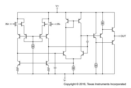
Figure 47. Equivalent Schematic (Single-Channel)
