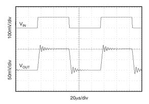
Figure 44. OPA827 Driving 2.2-µF Ceramic Capacitor
