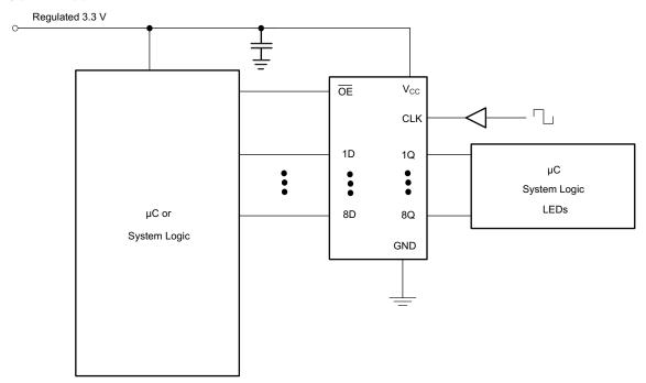
Figure 4. Typical Application Diagram
