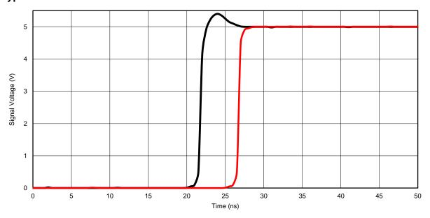
Figure 1. Response Time vs Output Voltage ( $T_A = 25$ °C,  $V_A = 5$  V)
