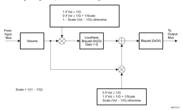
Figure 46. Biquad Gain-Control Structure
