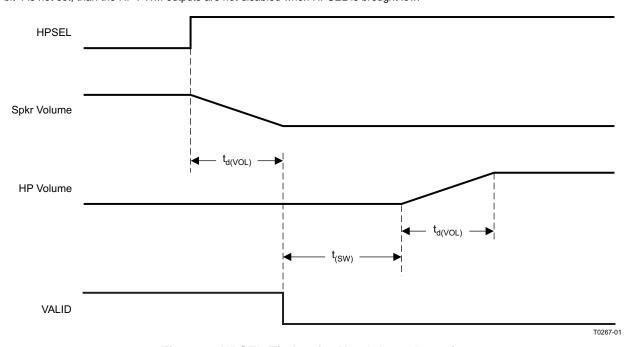
Figure 8. HPSEL Timing for Headphone Insertion
