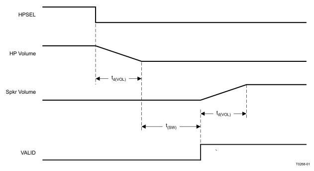
Figure 9. HPSEL Timing for Headphone Extraction
