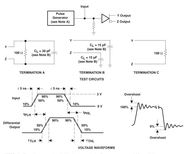
NOTES: A. The pulse generator has the following characteristics:  $Z_O$  = 50  $\Omega$ ,  $t_W$  = 25 ns, PRR  $\leq$  10 MHz.
