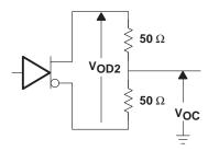
Figure 1. Differential and Common-Mode Output Voltages
