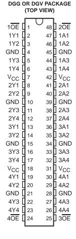
The device can be used as four 4-bit buffers, two 8-bit buffers, or one 16-bit buffer. It provides inverting outputs and symmetrical active-low output-enable (OE) inputs.
