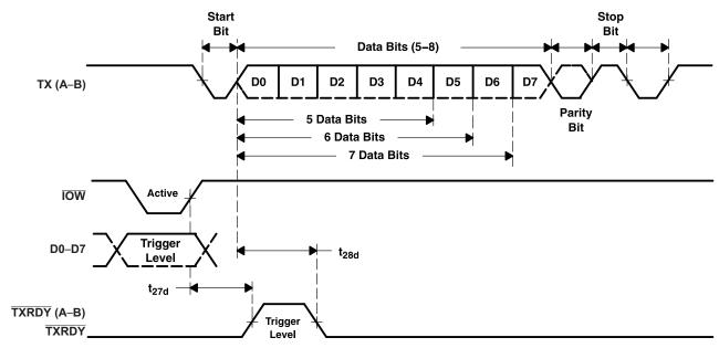
Figure 23. Transmit Timing in FIFO Mode
