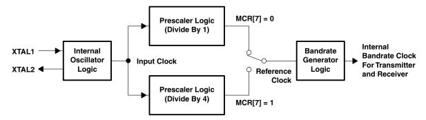
Figure 9. Prescaler and Baud Rate Generator Block Diagram
