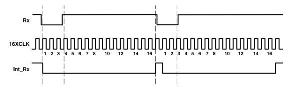
Figure 33. Timing Causing 1-Clock-Wide Pulse Between Consecutive Ones
