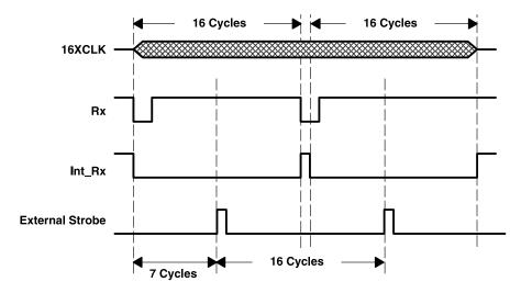
Figure 34. Recommended Strobing for Decoded Data
