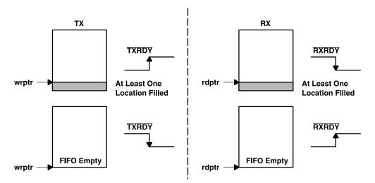
Figure 7. TXRDY and RXRDY in DMA Mode 0 or FIFO Disable
