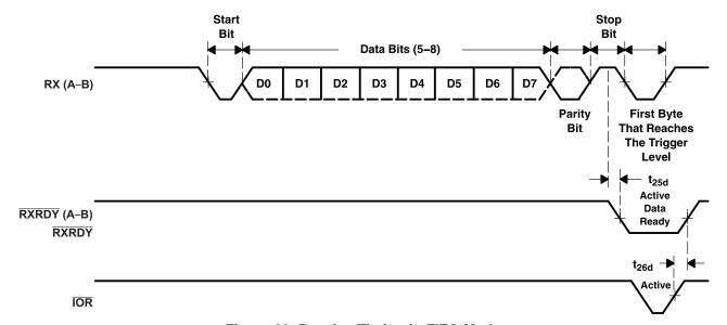
Figure 20. Receive Timing in FIFO Mode
