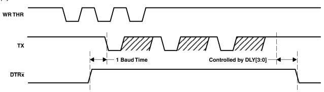
A. Waveforms are not shown to scale, as the WR THR pulses typically are less than 100 ns, where the TX waveform varies with baud rate but is typically in the microsecond range.
