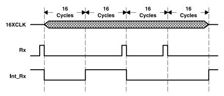
Figure 36. Positive Rx Pulse Decode – Macro View
