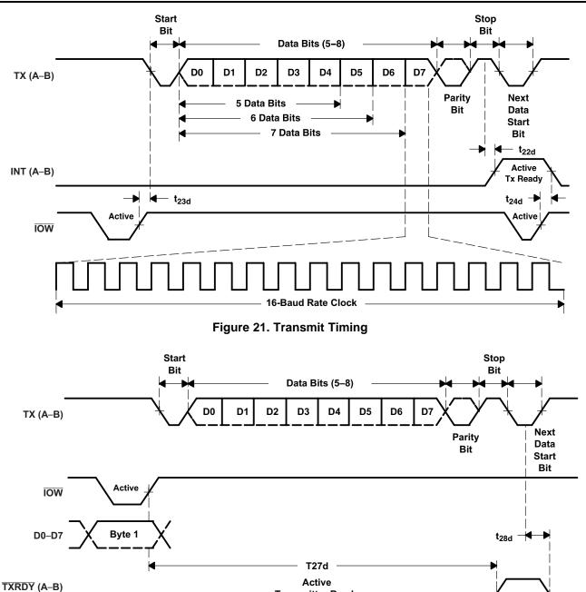
Figure 22. Transmit Ready Timing in None FIFO Mode
