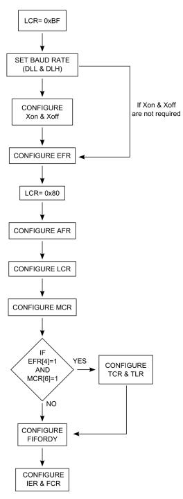
Figure 37. Diagram of the Generic Configuration Process
