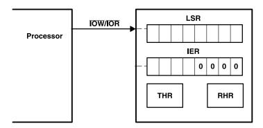
Figure 6. FIFO Polled Mode Operation
