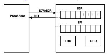
Figure 5. Interrupt Mode Operation
