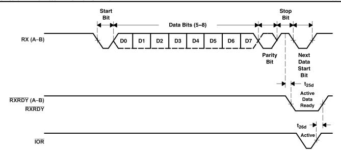
Figure 19. Receive Ready Timing in None FIFO Mode
