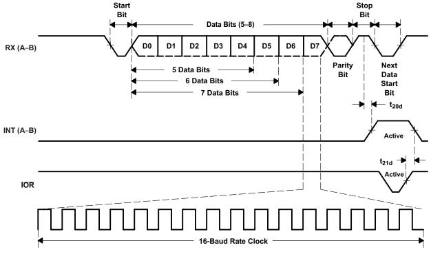
Figure 18. Receive Timing
