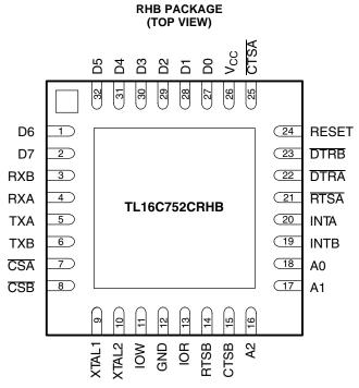
NOTE: The 32-pin RHB package does not provide access to  $\overline{DSRA}$ ,  $\overline{DSRB}$ ,  $\overline{RIA}$ ,  $\overline{RIB}$ ,  $\overline{CDA}$ , and  $\overline{CDB}$  inputs or  $\overline{OPA}$ ,  $\overline{OPB}$ ,  $\overline{RXRDYA}$ ,  $\overline{RXRDYB}$ ,  $\overline{and}$   $\overline{TXRDYA}$  outputs.
