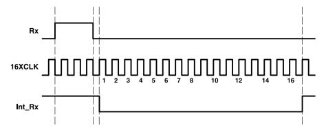
Figure 35. Positive Rx Pulse Decode - Detailed View
