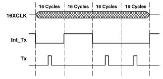
Figure 29. IrDA-SIR Encoding Scheme – Detailed Timing Diagram
