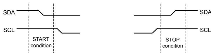
Figure 16-3. START and STOP Conditions
