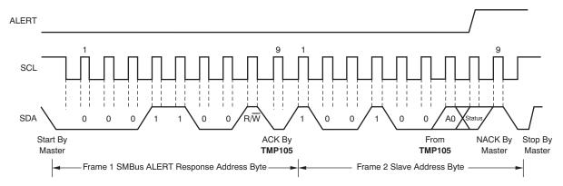
Figure 7. Timing Diagram for SMBus ALERT
