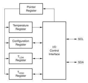
Figure 2. Internal Register Structure of the TMP105
