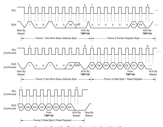
Figure 6. Two-Wire Timing Diagram for Read Word Format
