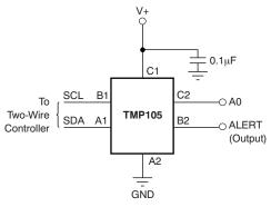
Note: SCL, SDA, and ALERT pins require pull-up resistors.
