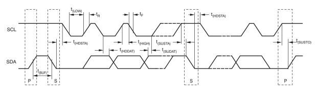
Figure 4. Two-Wire Timing Diagram
