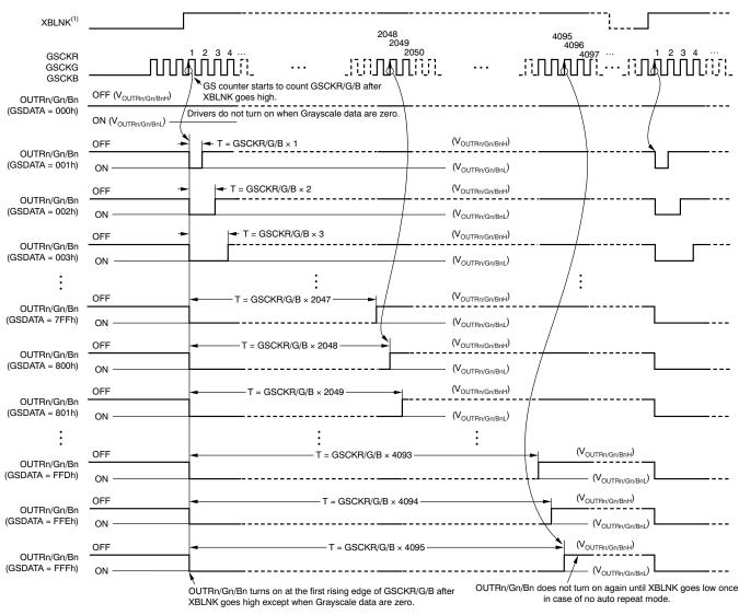
(1) The internal blank signal is generated when GSLAT is input for GS data with display timing reset enabled. Also, the signal is generated at 4096th GSCKR/G/B when the auto repeat mode is enabled. XBLNK can be connected to VCC when the display timing reset or auto repeat is enabled.
