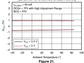
CONSTANT-CURRENT ERROR vs AMBIENT TEMPERATURE (Channel-to-Channel, BLUE Color)
