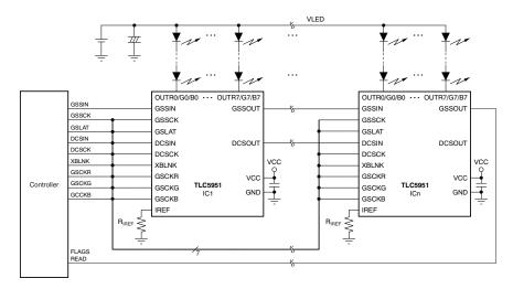
Typical Application Circuit (Multiple Daisy-Chained TLC5951s)
