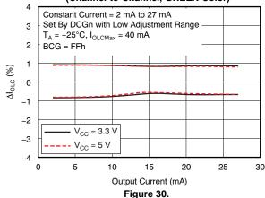
CONSTANT-CURRENT ERROR vs OUTPUT (Channel-to-Channel, BLUE Color)
