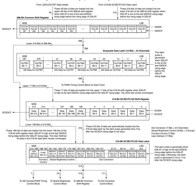
Figure 44. Grayscale Shift Register and Data Latch Configuration
