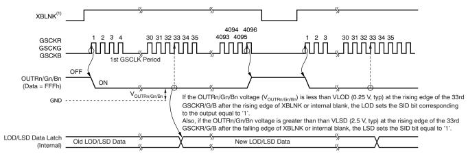
(1) The internal blank signal is generated when GSLAT is input for GS data with display timing reset enabled. Also, the signal is generated at the 4096th GSCK when auto repeat mode is enabled. XBLNK can be connected to VCC when the display timing reset or auto repeat is enabled.
