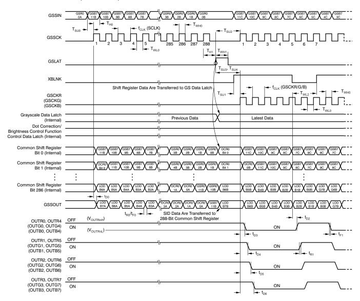
Figure 10. Grayscale Data Write Timing
