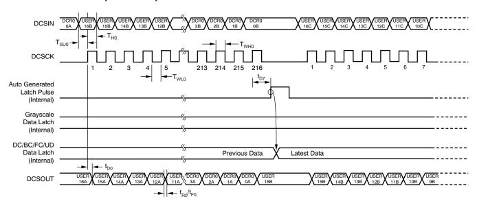
Figure 12. Dot Correction/Global Brightness Control/Function Control
