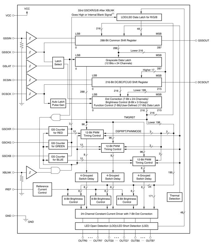
(1) The internal blank signal is generated when GSLAT is input for GS data with display timing reset enabling. Furthermore, the signal is generated at the 4096th GSCK when auto repeat mode is enabled. XBLNK can be connected to  $V_{CC}$  when the display timing reset or auto repeat is enabled.
