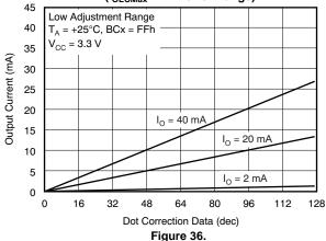
DOT CORRECTION LINEARITY (I<sub>OLCMax</sub> with Upper and Lower Range)
