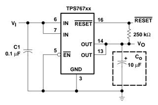
Figure 26. Typical Application Circuit (Fixed Versions)
