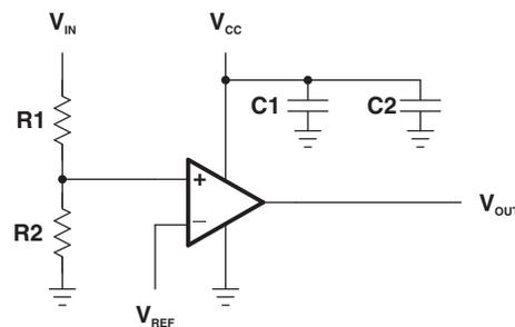
Figure 1. Threshold Detector
