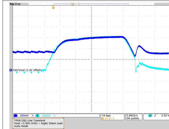
Figure 43. TPS61281A Forced Pass-Through to Boost Mode Transition
