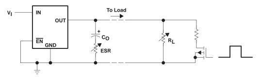
Figure 18. Test Circuit for Typical Regions of Stability (Figure 19)
