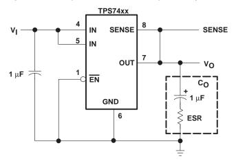
Figure 20. Typical Application Circuit
