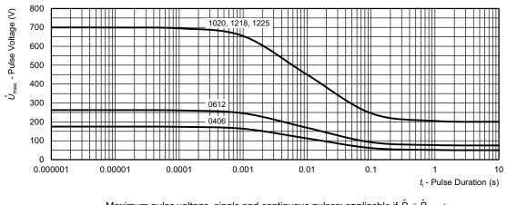
Maximum pulse voltage, single and continuous pulses; applicable if  $\hat{P} \leq \hat{P}_{max}$ ; for permissible resistance change equivalent to 8000 h operation
