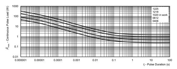
Maximum pulse load, continuous pulses; applicable if  $\overline{P} \le P(g_{amb})$  and  $\hat{U} \le \hat{U}_{max}$ ; for permissible resistance change equivalent to 8000 h operation
