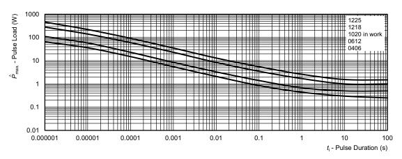
Maximum pulse load, single pulse; applicable if  $\overline{P} \rightarrow 0$  and n < 1000 and  $\hat{U} \leq \hat{U}_{max}$ ; for permissible resistance change equivalent to 8000 h operation
