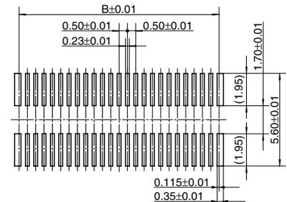
\* See the dimension table on page 5 for more information on the B dimension of the socket and header.
