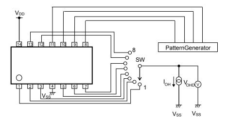
Figure 3. Test Circuit of Output H Voltage
