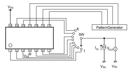
Figure 4. Test Circuit of Output L Voltage
