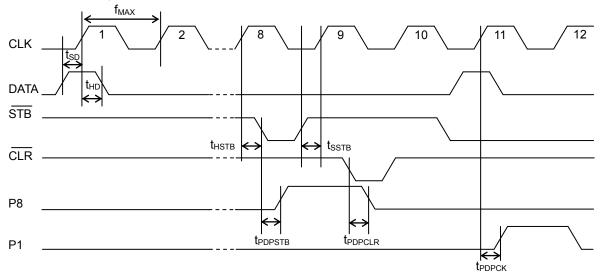
Figure 1. Waveform of Switching Characteristics
