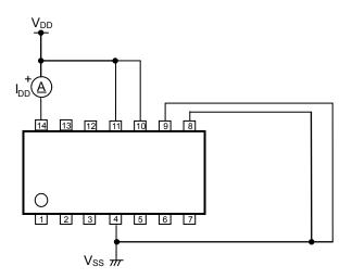
Figure 5. Test Circuit of Static Dissipation Current
