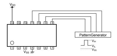
Figure 2. Test Circuit of Input H/LVoltage
