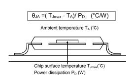
Figure 8. Thermal resistance
