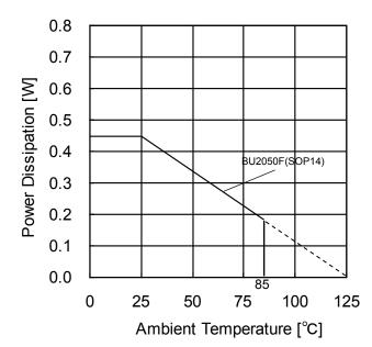
Figure 9. Derating Curve
