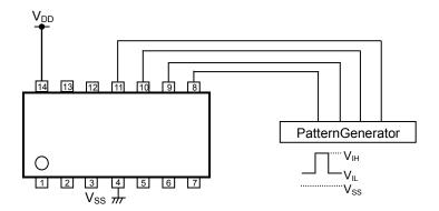
Figure 6. Test Circuit of Switching Characteristics
