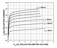
Figure 1. Static Characteristic
