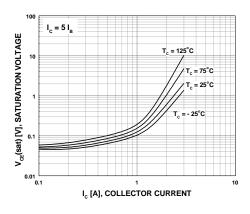
Figure 3. Saturation Voltage
