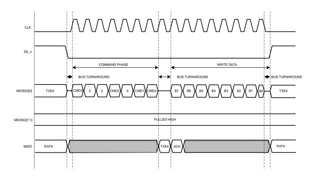
Figure 8.2 FT1248 1- bit write timing diagram
