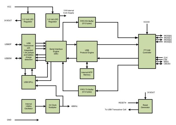
Figure 2.1 FT220X Block Diagram
