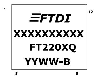
Figure 10.4 QFN-16 Package Markings
