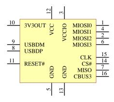
Figure 3.2 SSOP Schematic Symbol
