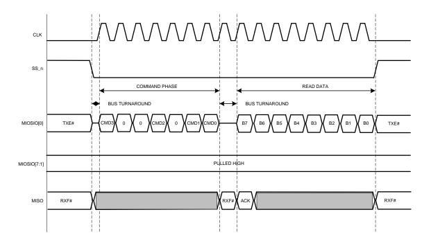
Figure 8.3 FT1248 1- bit read timing diagram
