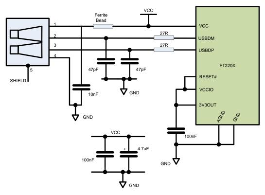
Figure 7.1 Bus Powered Configuration
