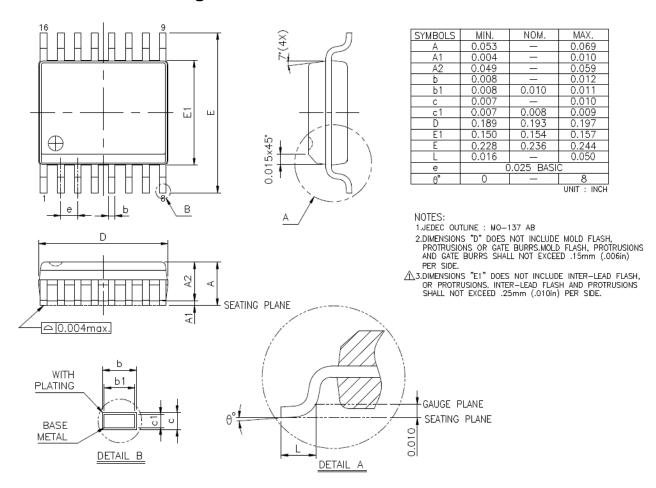
Figure 10.1 SSOP-16 Package Dimensions
