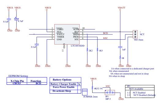
Figure 7.4 USB Battery Charging Detection
