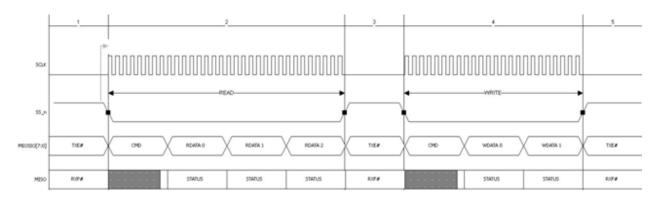
Figure 5.1: FT1248 Basic Waveform Protocol.
