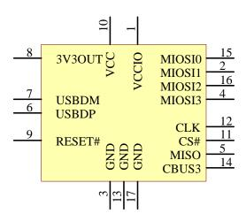
Figure 3.1 QFN Schematic Symbol
