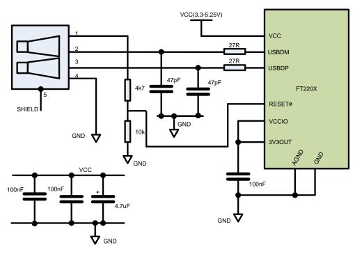
Figure 7.2 Self Powered Configuration
