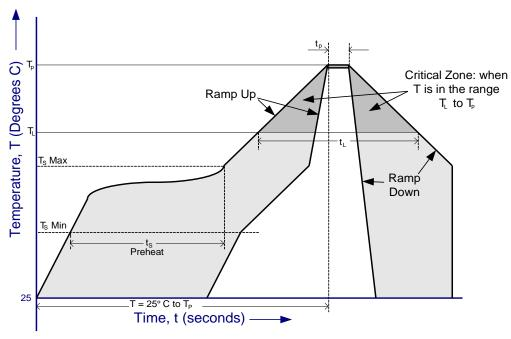
Figure 10.5 FT220X Solder Reflow Profile
