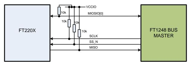
Figure 8.1 Application Example showing USB to FT1248 host
