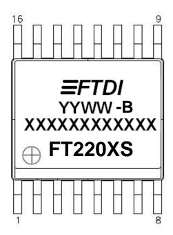
Figure 10.2 SSOP-16 Package Markings
